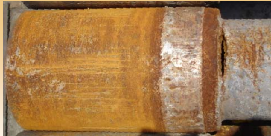
Piercing failure of drill pipe joint
