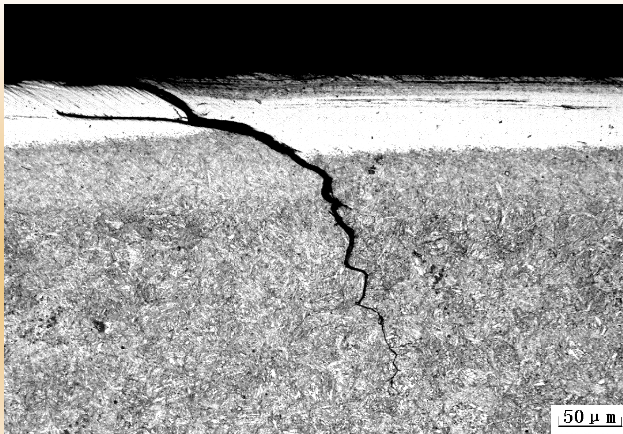
The microstructure of outer surface material of longitudinal fracture drill pipe joint
