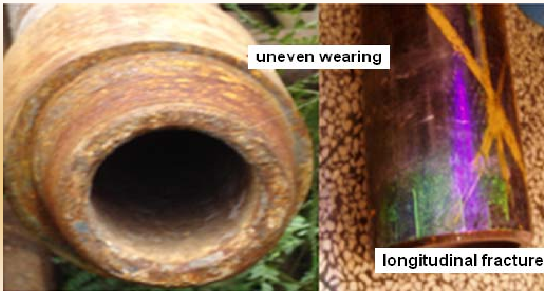
The uneven wearing and longitudinal fracture of drill pipe joint
