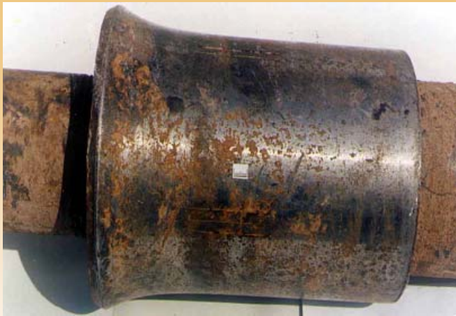
Expansion of drill pipe joint
